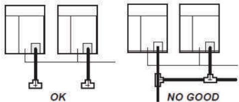
Y-shape branching joint for gas pipe
