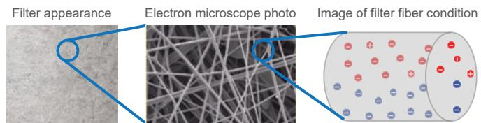
PM2.5 filter has "Electrostatic" solution.
