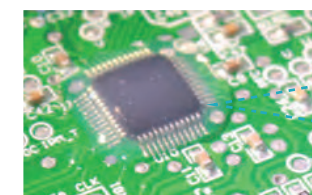
The surface of the control board uses surface mounting material
