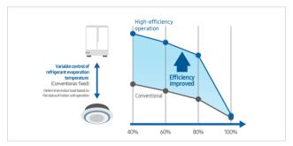
Improves the operation efficiency of air conditioners by controlling outdoor units' refrigerant evaporation temperature and compressor current according to the indoor load.
