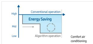
Prevents overcooling/overheating by calculating proper temperatures considering climate and human factors. (clothing, activity, etc.)
