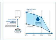
Improves the operation efficiency of air conditioners by controlling outdoor units' refrigerant evaporation temperature and compressor current according to the indoor load.
