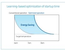
Saves energy by predicting the time to reach the target temperature based on data on temperature changes and air conditioning setting. • Efficient outdoor unit operations
