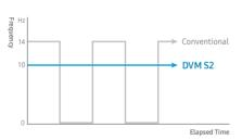
The Active Frequency Drive of the Samsung DVM S2 enables the compressor to operate at the lowest revolution of 10Hz, which prevents the operation from frequently turning on and off, so it maintains the indoor temperature more precisely to ensure continuous comfort.
