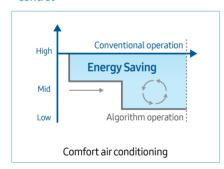
Prevents overcooling / overheating by calculating proper temperatures considering climate and human factors. (clothing, activity, etc.)
