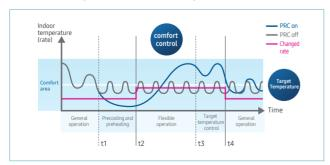
Reduces energy consumption and operating costs by controlling indoor temperature and outdoor unit performance to respond to the time-varying rate system.
