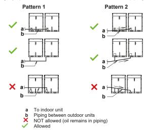
To avoid the risk of oil retention to the outmost outdoor unit, always connect the stop valve and the piping between outdoor units as shown in the correct (
