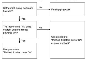
It is very important that all refrigerant piping work is done before the units (outdoor, SV unit or indoor) are powered on. When the units are powered on, the expansion valves will initialise. This means that the valves will close.
