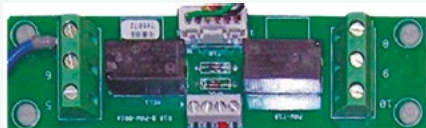
T10 interface PCB with digital and relay connections.
