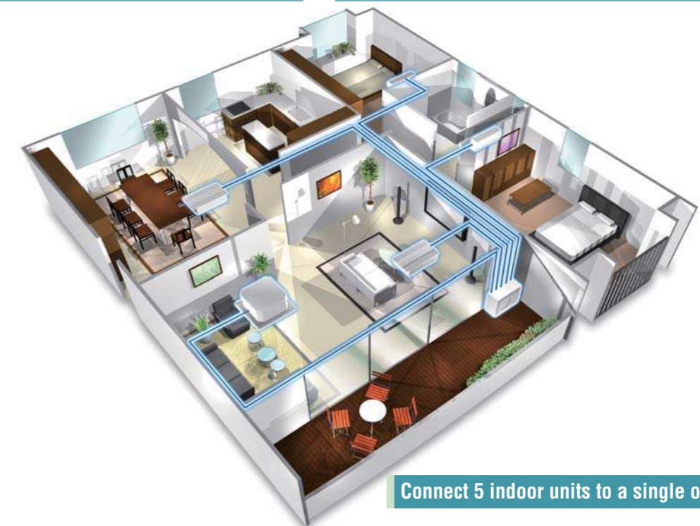
Up to 5 indoor units can be connected.
