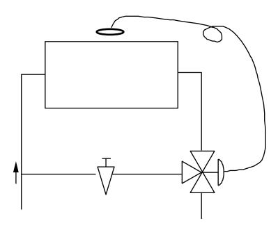
Variable flow through coil Constant flow through system
