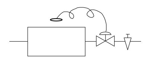
Variable flow through coil Variable flow through system
