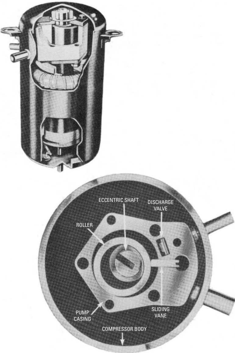
Figure 9-6 Eccentric shaft and roller of a rotary compressor. (Courtesy Mueller Climatrol Corp.)
